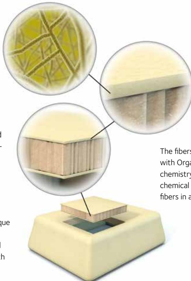
The fibers are linked together with OrganoClicks click chemistry establishing strong chemical bonds between the fibers in a dense matrix.
