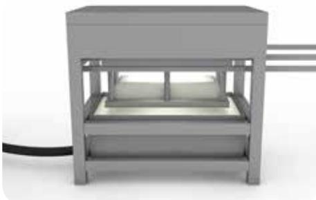
3. The male tool is lifted up with the fibers attached to the surface of the tool.
