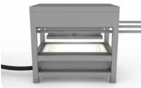
4. The male tool is pressed into the female tool under high pressure. The female tool is equipped with heating and a vapor transmission system that moulds the fiber mixture into a form-stable 3D shaped biocomposite object.
