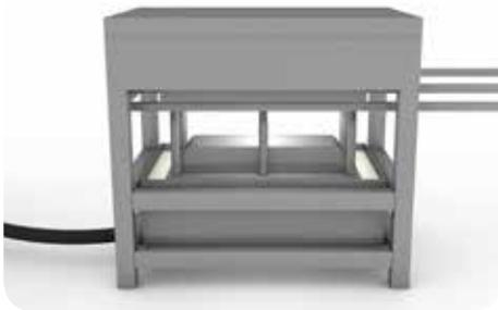
1. A perforated male aluminum tool is connected to a vacuum system.
