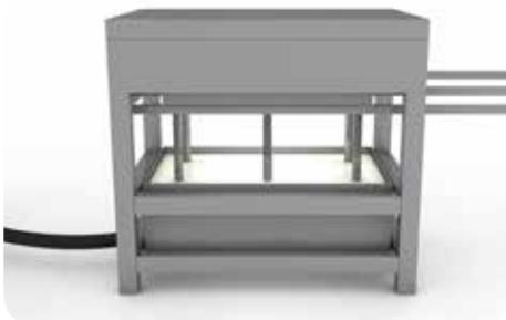
2. The male tool is submerged into a mixture of biofibers that are functionalized with OrganoClicks different technologies in order to achieve the right properties. Vacuum is applied. The fibers stick to the tool.
